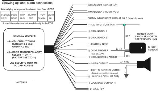
NOTE: THE M40 HAS ONLY ONE TRIGGER INPUT FOR BONNET, BOOT, DOORS AND SHOCK SENSOR. CONNECT THE BOOT SWITCH TO A REAR DOOR AND ADD DIODES AS SHOWN.
