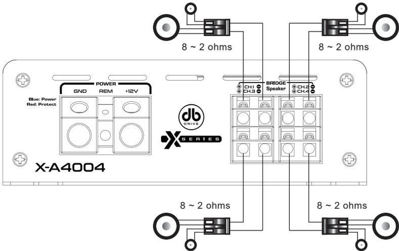
3-6B. X-SERIES 4 CHANNEL AMPLIFIERS' SPEAKER CONNECTION DIAGRAM 2.
